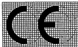
— If the CE marking is reduced or enlarged the proportions given in the above graduated drawing must be respected.
